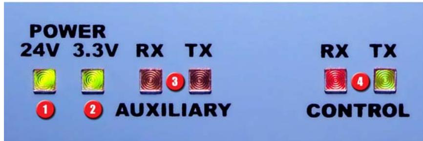
1. Power Indicator Light 1 (24v dc). When illuminated indicates the 24v input power is adequate. When off indicates the 24v input power is below the required specification (Approximately 23.3 v). The 24v input power supplies power to all connected Smarteye readers and the Netx internal electronics.
