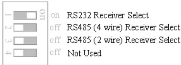
Note: RS232 or RS485 can be selected but not both. Switch SW2 must be set to match
